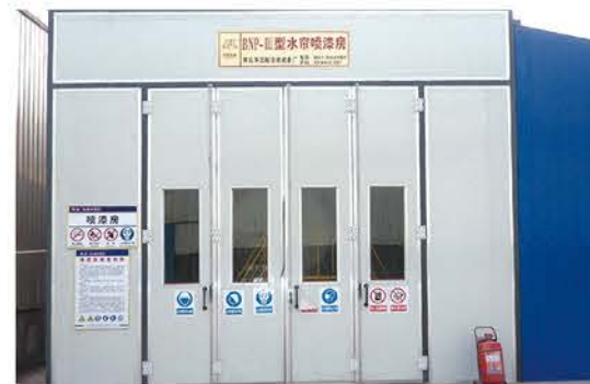
Water curtain type spray booth
