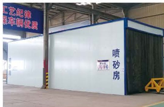
Shot blasting and powder coating booth
